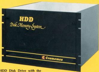
Combining the new Model HDD Disk Drive with the Cromemco System Two Computer gives you a fast, powerful system with a Z-80A microprocessor, two floppy disk drives, up to 512 kilobytes of RAM and up to 22 megabytes of hard disk storage.
